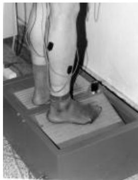
**Figure 1** The trap door used to cause the inversion perturbations of the ankle joint when the subjects stand on it.
