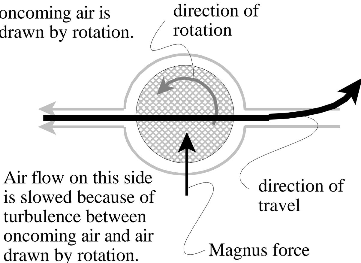
Air flow on this side is slowed because of turbulence between oncoming air and air drawn by rotation.
