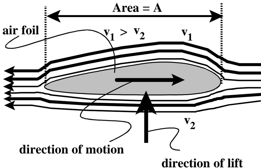
$$F_{lift} = C_{lift} \rho A_p v^2$$
